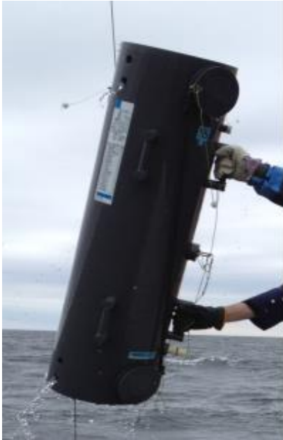
A 60 L GO-FLO bottle used to obtain large sample volumes for carbon-14 analysis of seawater methane. Two such bottles were used in parallel during the expedition.
