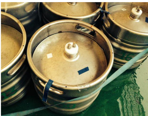
Kegs ready for sampling of seawater for storage and stripping back at ITM. Some kegs have stubs instead of the normal tubing of the headpieces. Others have white plastic screwtop lids. They are all marked with blue tape at the handle, with the text "ZnCl 2 ".
