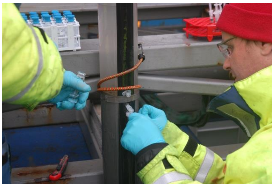
Figure F. 2.6.2 Sediment methane sampling through core liner
