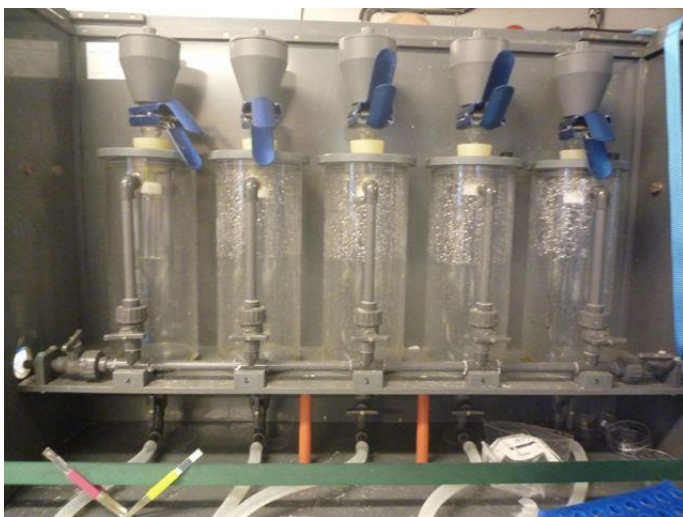
Vacuum filter system used for small-volume GF/F filtration. Five parallel filter devices are hooked up to the same vacuum source.
