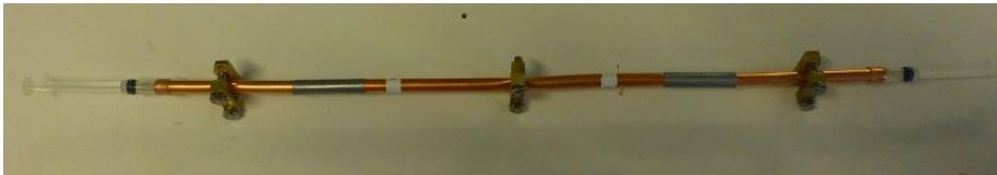
A copper tube of the type used for sampling for helium isotopes in seawater.
