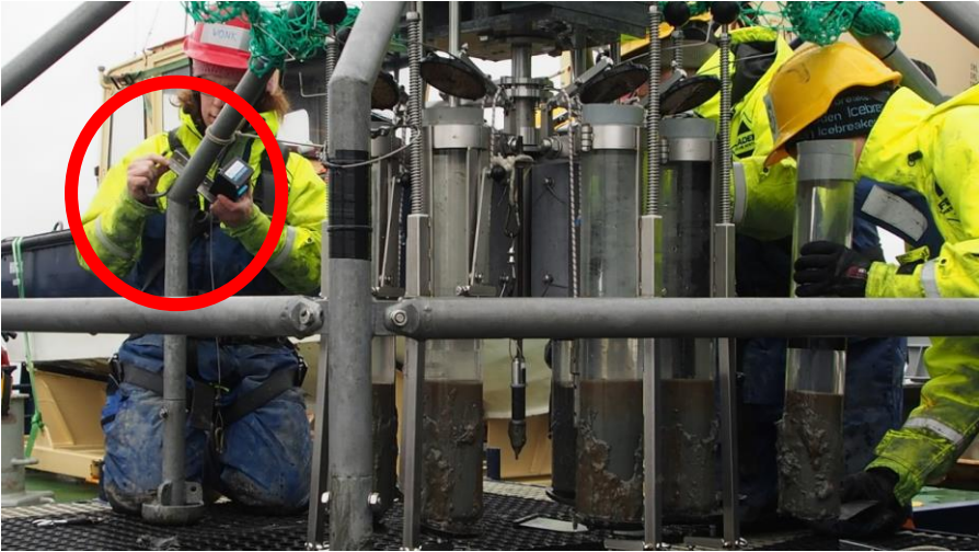
Figure E.8. Underwater camera being mounted
