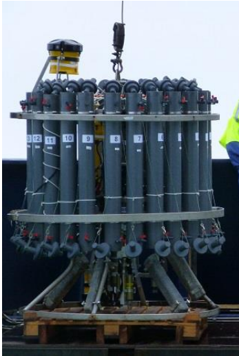
The CTD rosette with 24 Niskin bottles, here ready to be deployed from the forward A-frame.
