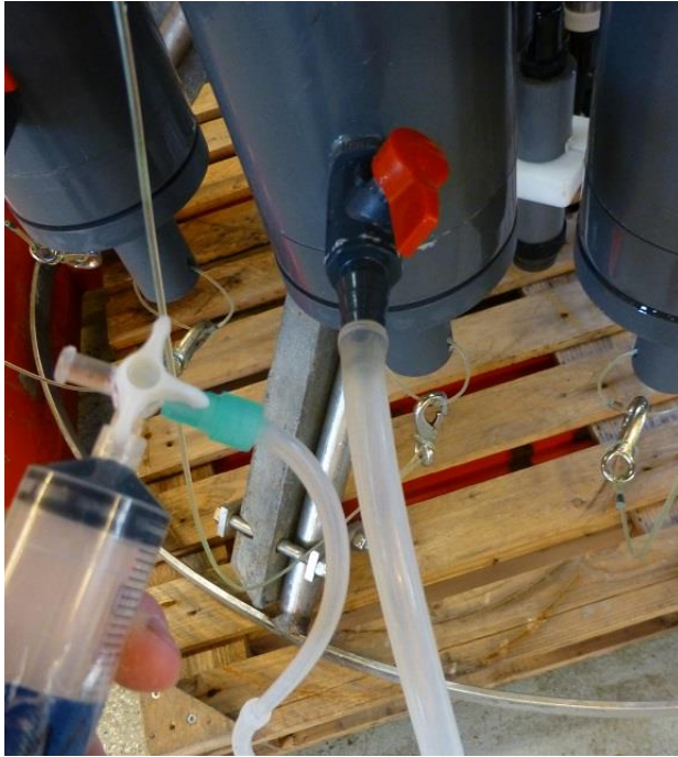
Subsampling from a Niskin bottle to 60 mL syringe using a silicon tube and a 3-way valve.
