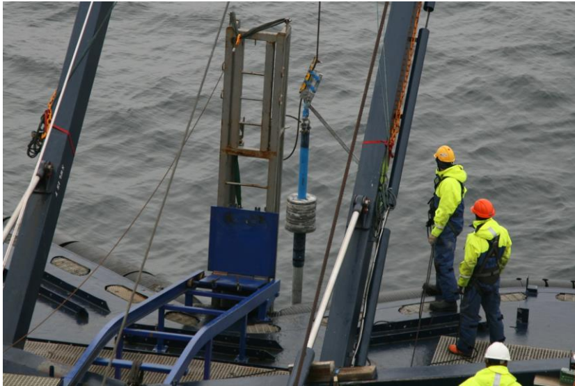
Figure E.3. Piston corer during deployment
