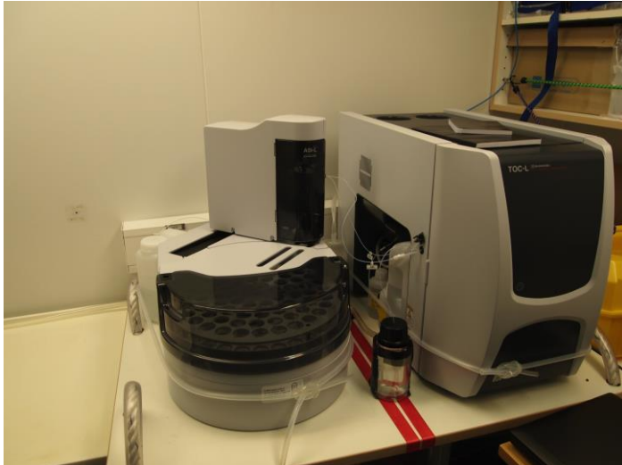
Shimadzu TOC-L total organic carbon analyser with autosampler (left) in the clean lab on board ODEN.
