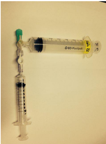
The two types of syringes used for the headspace extraction and the injection to GC. Note how the two valves are attached with Luer-Lock fittings to each other for flushing with, and transfer of, headspace.
