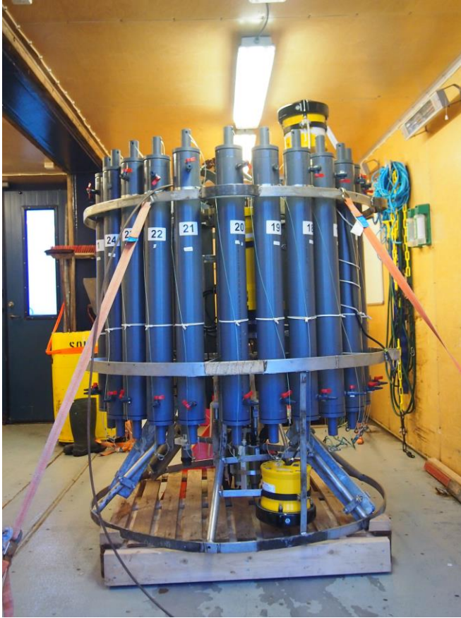
Figure G1. The rosette setup with the upward and downward looking ADCPs (yellow casing) .
