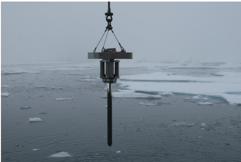
Figure E.2. Rumohr corer after deployment
