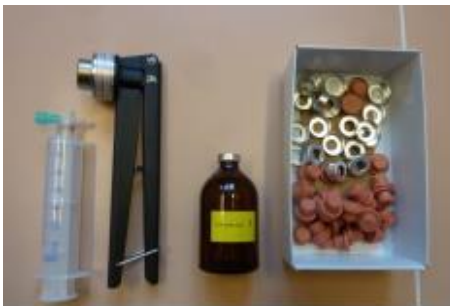
Examples of the 60 mL plastic syringe, 120 mL serum bottle, stoppers, crimp caps and crimp tool used during sampling from all sampling platforms.
