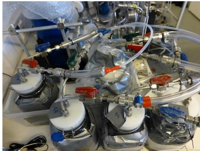
Four sediment jars connected in series with an empty jar (serving as "dirt trap") for stripping of CH 4 in sediment.
