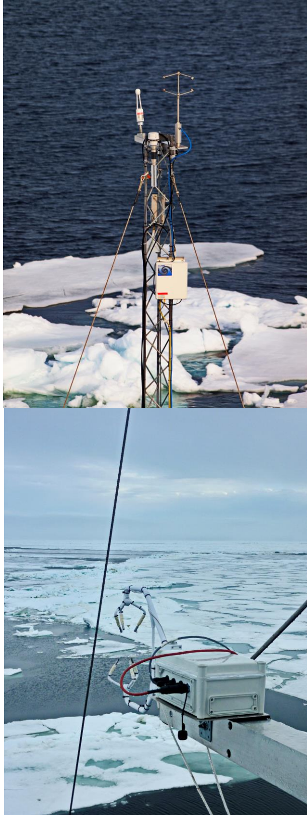
Figure MT2. Photos of the turbulence/surface flux instruments with (left) the top Metek/Licor/CLASP instrumentation with its motion sensor, and (right) the CSAT sonic on its retractable boom with the motion sensor mounted.
