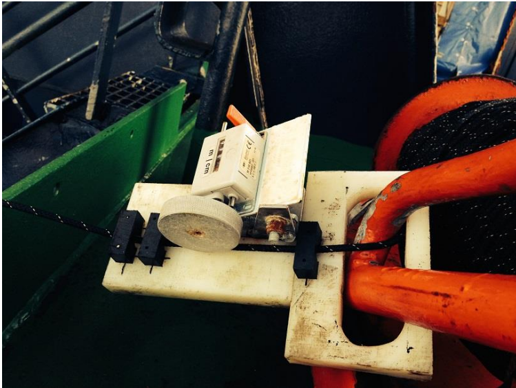
The metering wheel for the red winch, sitting on the wire handle (used to feed the line properly onto the drum).
