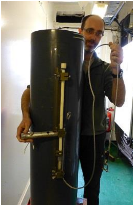
A GO-FLO bottle with mounted wire for quick switch between GO-FLO bottles on the Red Winch Kevlar line. A weight of 15-20 kg was attached to the wire during operation. Also note the tool used to quickly open/fasten the weldment wing nuts (a pipe with a matching slot in it).
