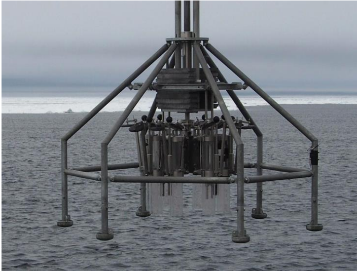
Figure E.1. Multicorer during deployment
