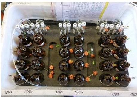
Two “kit boxes” like this were used to prepare and organize sampling vials, stoppers with needles through them, sub-sampling tube, our own decksheet, and 60 mL plastic syringes. This was a great help, considering that five to six sample types were taken from every Niskin bottle.
