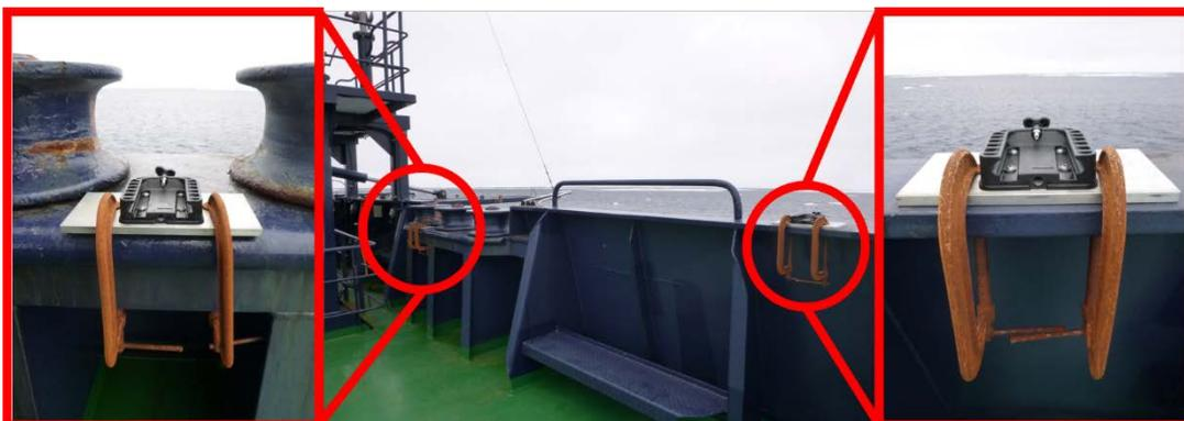
*Figure 4. Detail of bow reel mounts. Mount on left is center bow mount for securing bow reel throughout deployment and calibration; mount on right is starboard bow mount for temporarily securing starboard reel during line deployment and port line movement.*
