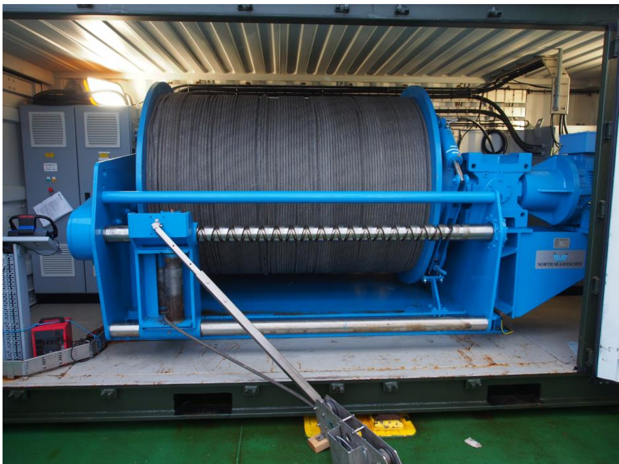
Figure SC-8: Coring winch manufactured by NorthSea.
