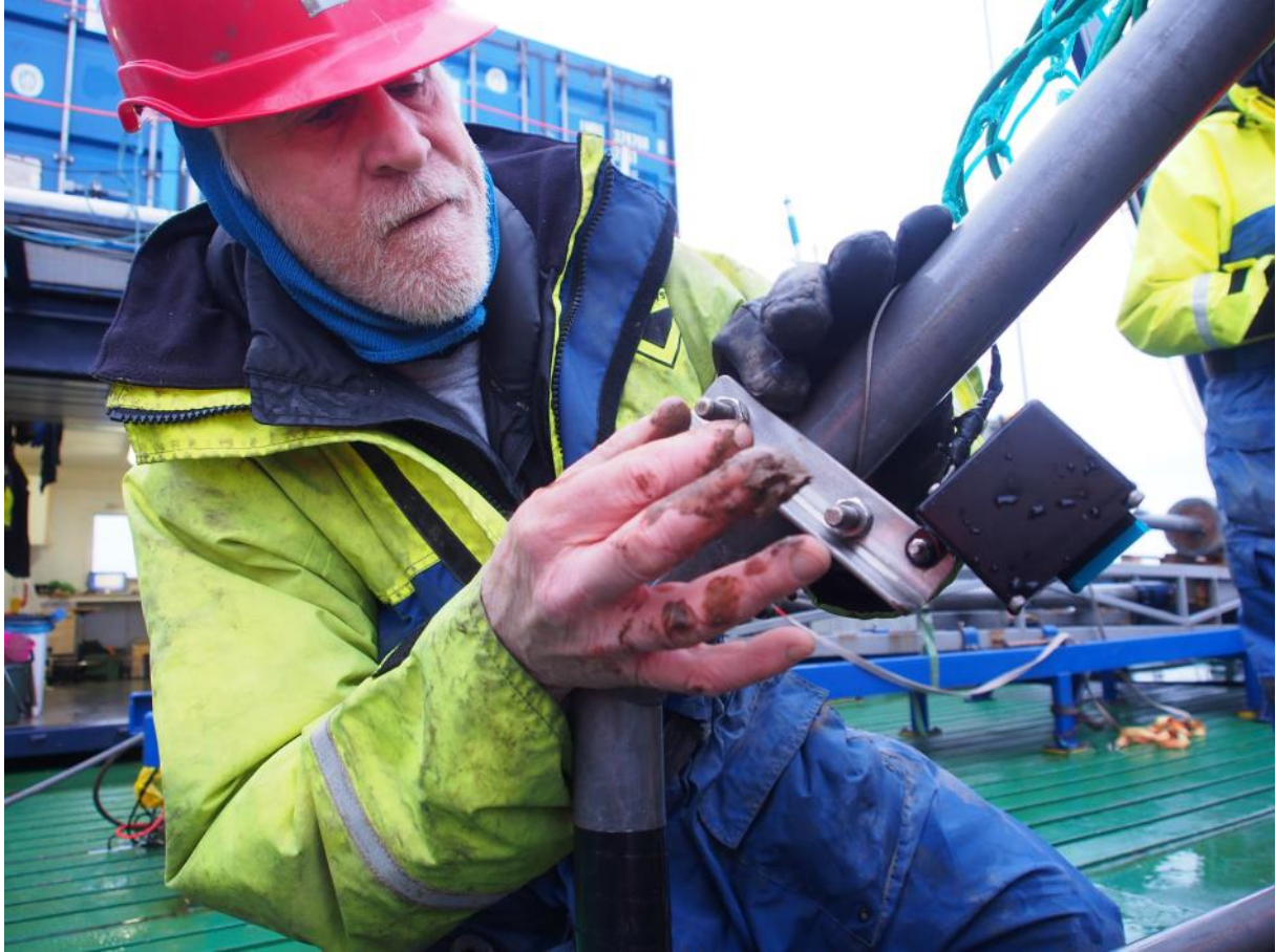
Figure SC-6: The GoPro Hero3+ camera mounted on the multicorer frame in the ScoutPro H3 housing.
