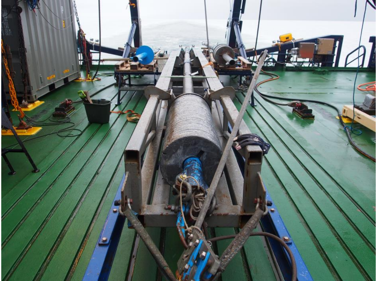
Figure SC-2: Stockholm University large diameter piston corer (center) resting in the deployment cradle. This large diameter corer can also be rigged as a gravity corer, seen to the right. The standard setup during Leg 2 of the SWERUS C3 cruise was to have both a gravity corer and a piston corer rigged and ready for deployment. In addition, the smaller diameter corer is seen to the left in this photo with a blue core head top. This smaller corer was only used once during Leg 2 to take a gravity corer at 1665 m water depth because the winch used could not handle the large diameter and heavier corer at depths deeper than approximately 1500 m (see winches).
