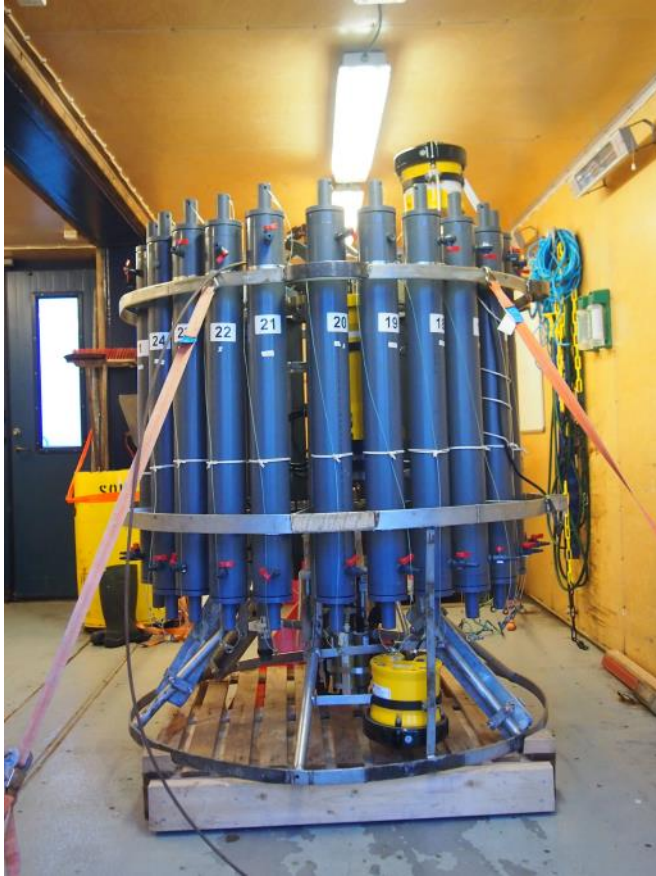
Figure PO-1: The rosette setup with the upward and downward looking ADCPs (yellow casing).
