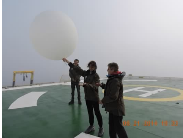
Figure BLM-4: Launch of a rawinsonde weather balloon during Leg 2.
