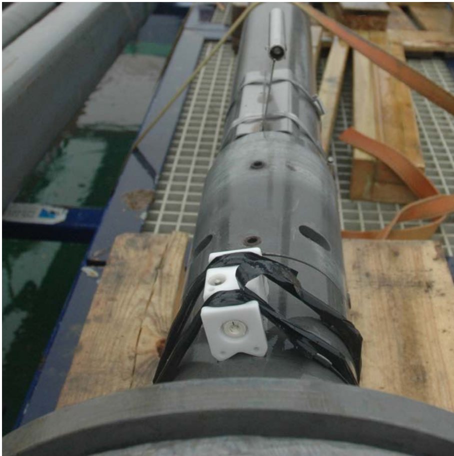
Figure PP-5: Position of the DSC magnetic sensor on the core barrel.
