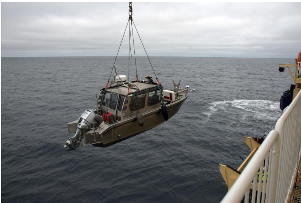
Figure GM-5: Launching of RV Skidbladner using IB Odens crane. Photo Arne Lif.
