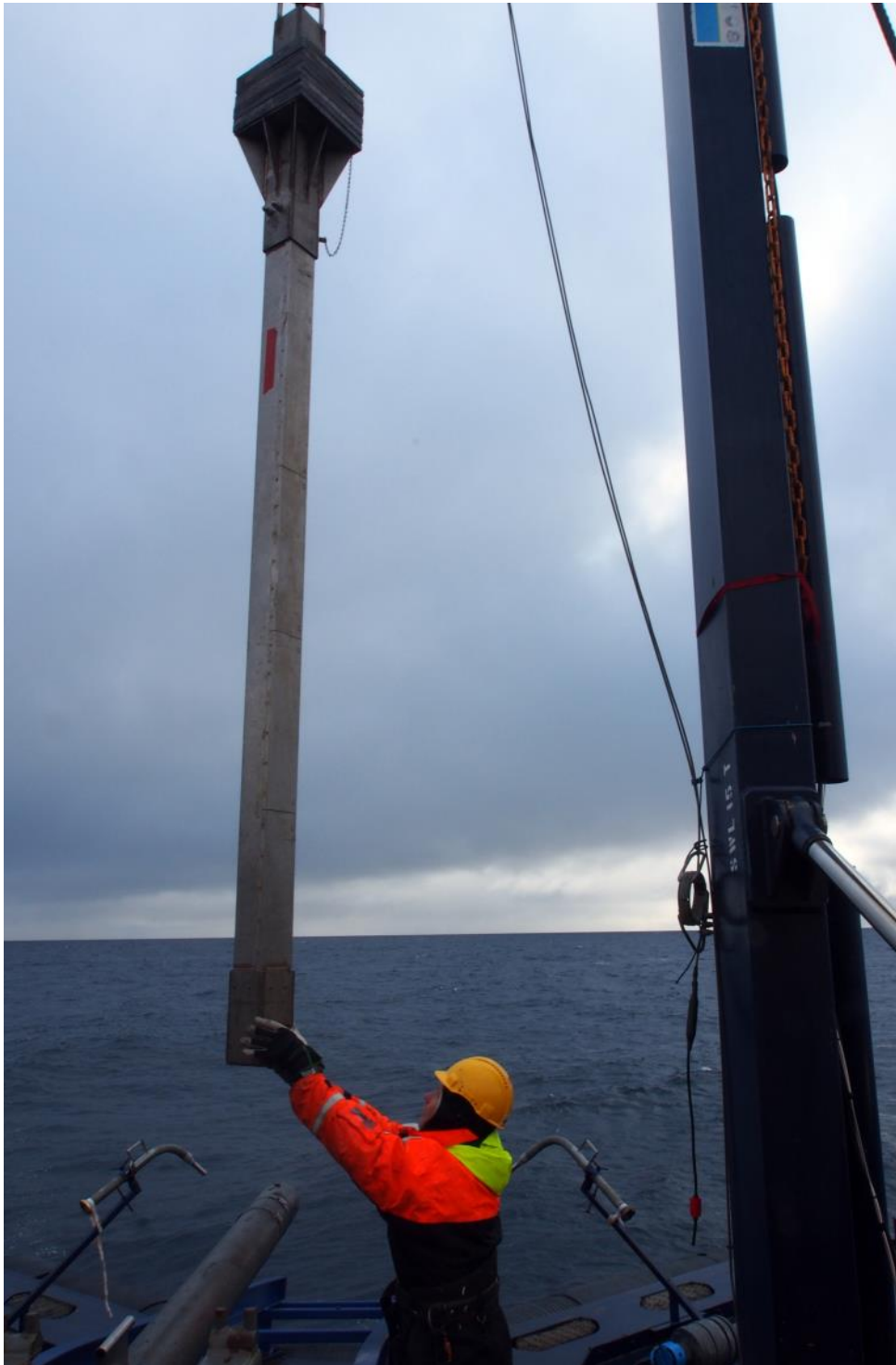
Figure SC-7: Kasten corer.
