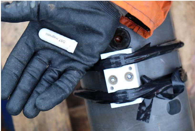
Figure PP-4: Star Oddi DSC magnetic sensor and casing attached to the core barrel.
