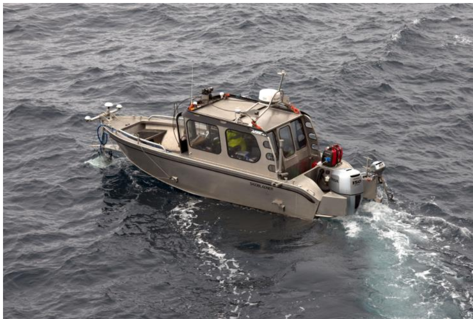
Figure GM-3: RV Skidbladner with the EM2040 bow mounted multibeam in operation in the Chukchi Sea. The multibeam and sub-bottom profiler can be hoisted up for fast transit if required. Photo: Arne Lif.
