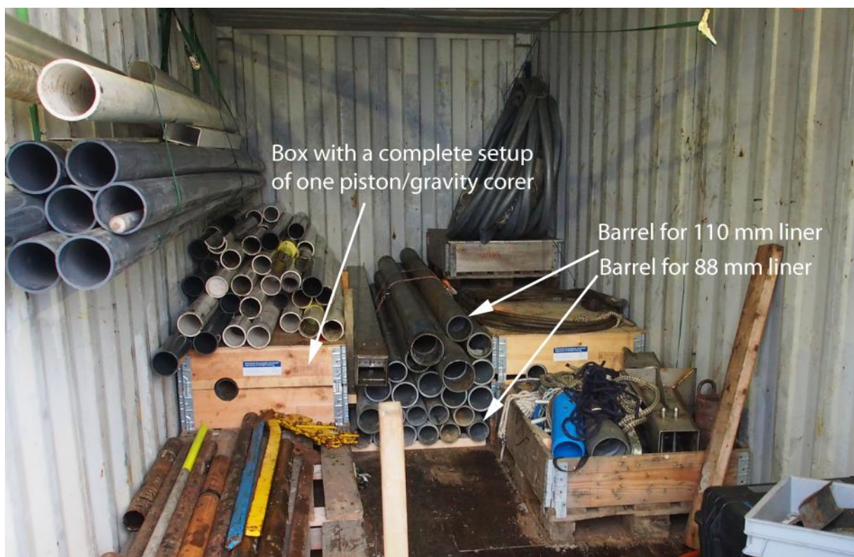
Figure SC-1: Container with the piston/gravity corer stored. Four complete setups were stored in this 20' container except for the lead weights and liners. The liners were made in 6 m long lengths to fit a multiple of 3 m, which is the length of each core barrel. This made the liners slightly too long to fit in a 20' container.
