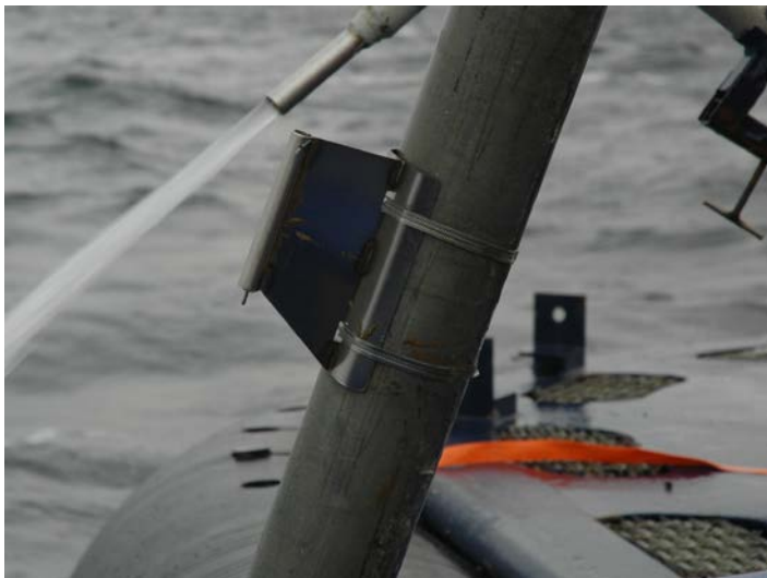
Figure PP-2. Stainless steel outrigger fins to attach the temperature probes to the core barrel.
