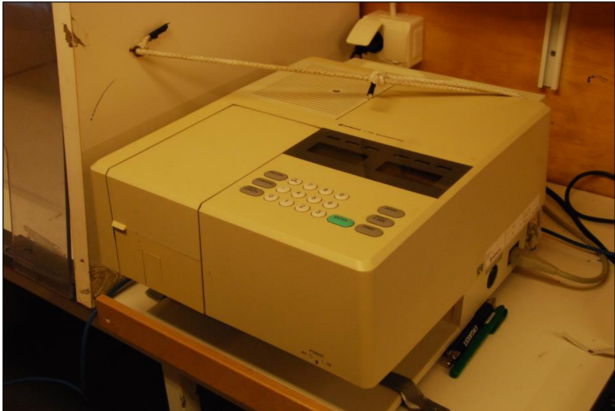
Figure CP-5: Spectrophotometer used for phosphate and ammonia analyses. Photo Clint Miller.
