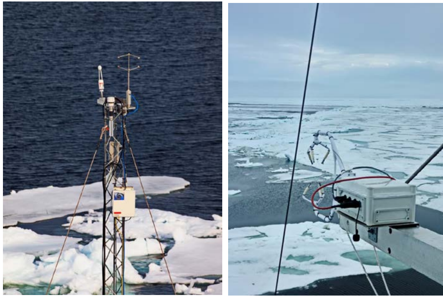
Figure BLM-5: Photos of the turbulence/surface flux instruments with (left) the top Metek/Licor/CLASP instrumentation with its motion sensor, and (right) the CSAT sonic on its retractable boom with the motion sensor mounted.
