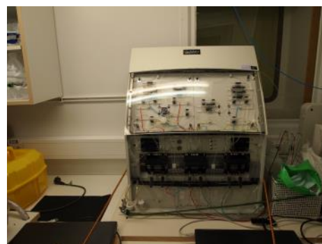
Continuous flow analyser QuAAtro from SEAL Analytical in the clean lab on ODEN. The instrument was used for continual on board measurements of nutrients in water throughout Leg 2.
