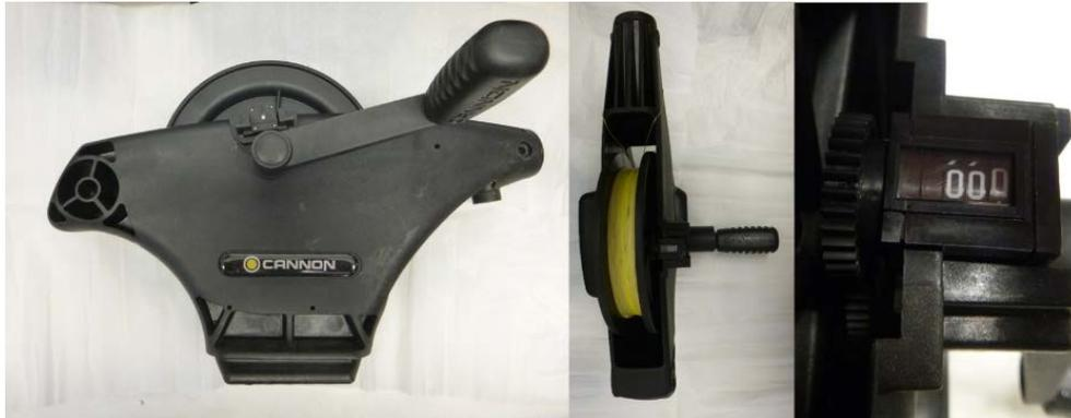
*Figure 3. Detail of deep sea reel ('downrigger') and counter.*
